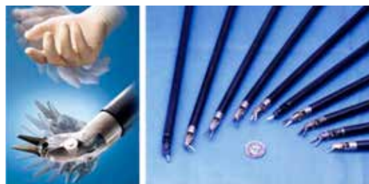
Fig 4: Repertoire of da Vinci® robotic instruments and their range of movement compared with the human wrist
